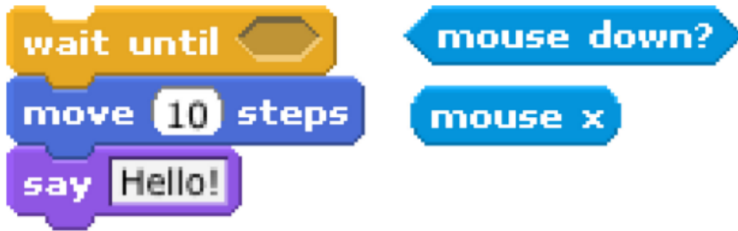
Fig. 5. Shapes indicate type. On the left, command blocks with parameter slots for boolean, number, and string parameters. On the right, boolean and number function blocks. (Maloney, 2010)
