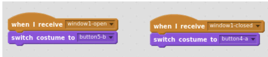
Image 2. Script for sprites reacting to the readings from GPIO pins Source: STEMKIT4Schools project
