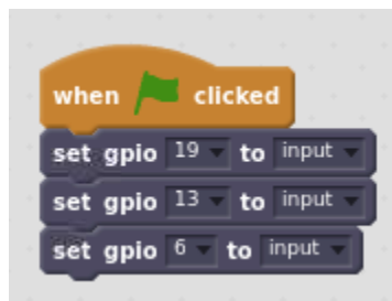
Image 3. Beginning of the code – setting relevant GPIO pins as input ones Source: STEMKIT4Schools project
