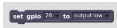
Image 9. Setting buzzer's GPIO to low after the main loop Source: STEMKIT4Schools project
